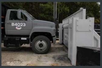
The gate design was then aesthetically enhanced by removing the front two support legs and independently tested by the Transport Research Laboratory (TRL) with a US truck (15,000lb truck at travelling at 50 mph) in accordance with the US Standard ASTM F 2656 ( supersedes DoS SD-STD-02.01) again the gate stopped the vehicle and zero penetration was achieved.
