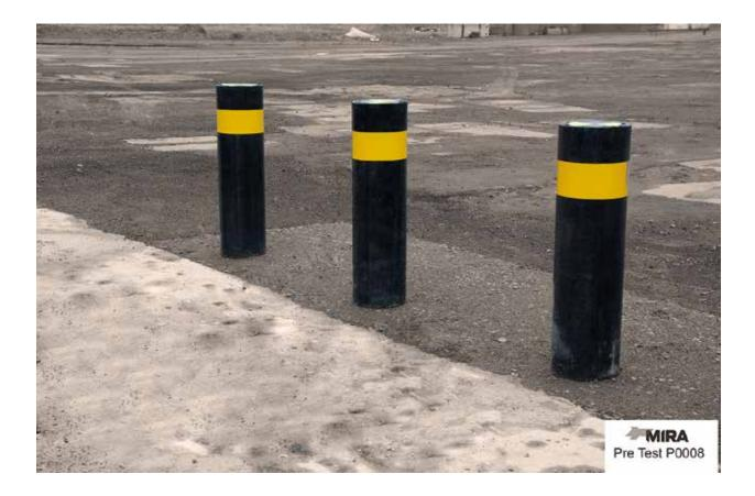
**The Avon Resilience SSF100 Bollard** is a super shallow foundation bollard, designed to provide stand-off hostile vehicle protection for infrastructure without the need for deep foundations.
