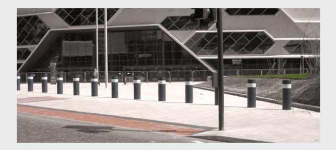
**Avon's Scimitar PAS 68 tested Static Bollards** provide a high level of security against unauthorised vehicle access without the need for an outwardly aggressive appearance.
