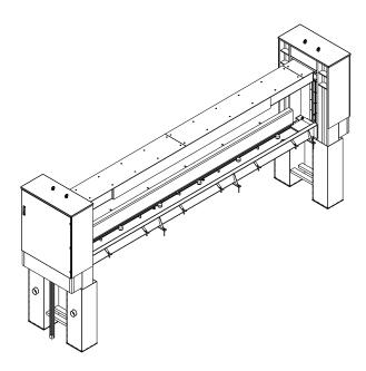
Design: Barrier Lift System with electro-hydraulic drive in separate drive cabinet,
